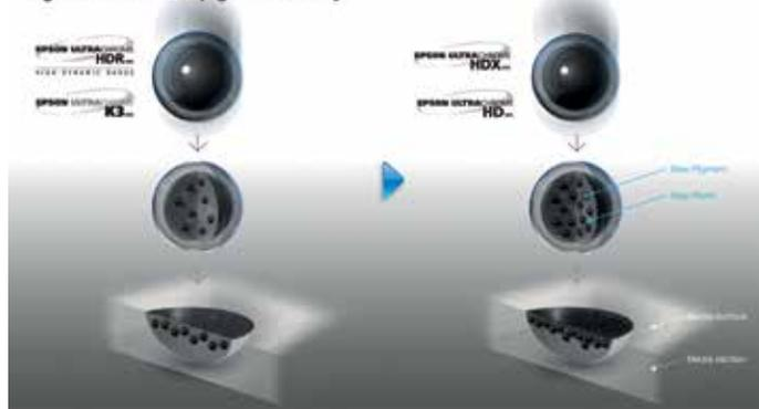
The proven Epson UltraChrome pigment inks offer smooth gradation and sharp definition, by utilising a three-level black ink technology that simultaneously employs black, light black and light light black ink to produce brilliant black density and grey balance. At the media surface, the UltraChrome HDX and HD matte and photo black inks achieve a much higher pigment density, ensuring the pigments do not penetrate too deeply when printing on third-party media.
