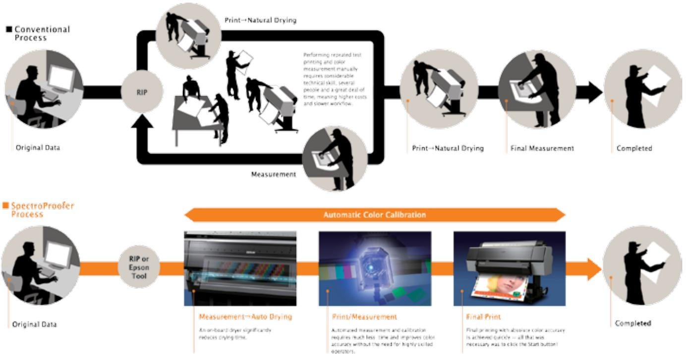
Available as an optional add-on, the ILS30 spectrophotometer (developed jointly with X-Rite) is essential to anyone who's looking for real efficiency in the proofing industry. It is capable of extreme measurement accuracy of below 0.2 dE-CMC. It simply attaches to the front of the printer, giving users the basis for an advanced colour management system.
